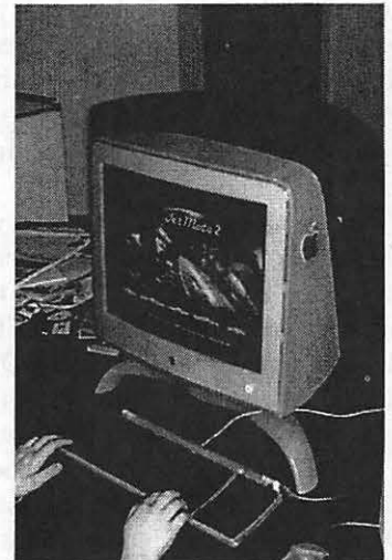
The new blue and white 17" Apple Studio Display (designed to match the new "Power Macintosh G3 blue and white") has a nice, sharp picture. Almost as impressive as the picture is what is on the screen: JetMoto2 , a Sony Playstation videogame, loaded from a CD-ROM and running on the Power Mac using Virtual Playstation, from Connectix. (Photo by Lawrence I. Charters)
