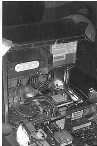
The inside of the new "Power Macintosh G3 blue and white" reveals an incredibly clean, accessible design: the computer opens right up, with almost no effort. The processor is under the cube-like heat sink at the bottom center, with the PCI video card standing behind it to the right. (Photo by Lawrence I. Charters)
