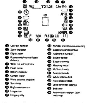
Figure 3 - Information presented on the monitor display. Nearly every conceivable tidbit about the exposure can be read out here. The data is superimposed on the image in playback mode. It can be suppressed by a single push of the "monitor" button.
