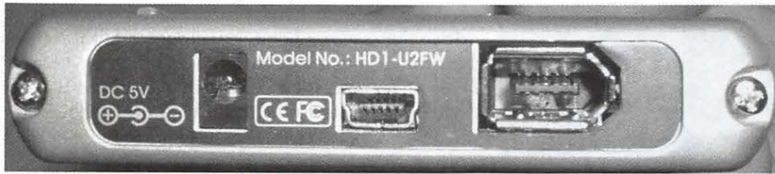
Figure 4 - Rear view of Hotdrive 2.5" Mobile showing external connections.
