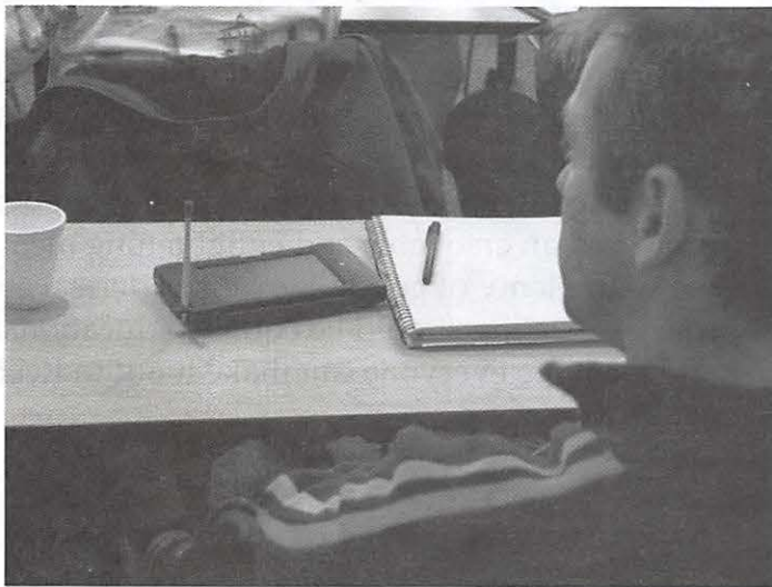
Figure 3 - One meeting attendee had this innovative portable computer. Battery powered, it accepted hand-written notes using the stylus, shown in a holder located right on the computer. What a wonderful idea!
