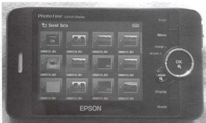
Figure 5 - When flash card media is read into the Epson P-4000, all photos imported on a given day are placed in a directory named after the year, month and day. If multiple cards are read on the same day, the folders are automatically numbered in the order they were imported
