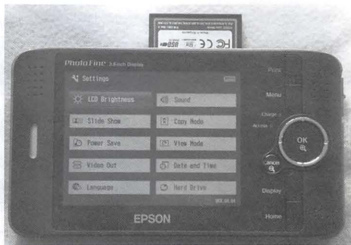
Figure 3 - Using the Settings menu, you can adjust the LCD brightness (shown selected in the photo), the sound volume, slide show options, copy modes, power saving modes, and a number of other details.
