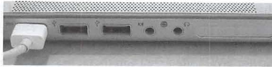
MacBook Pro ports, left side: Power connection, USB, USB, audio in, audio out, ExpressCard/34 slot.
