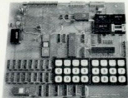
RS232 compatible. There are 12 quasi-bidirectional I/O lines with handshaking, and 14 more regular I/O lines, 5 heavy duty relays, and Teletype and audio cassette interfaces. All on one board.
