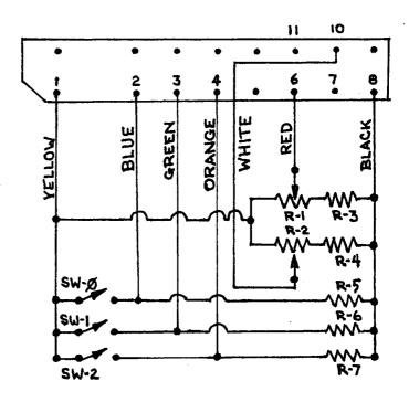
R1,2 - JOYSTICK, 100K LINEAR TAPER R3,4 - 360K, 1/4 WATT, 5% R5,6,7 - 1K, 1/4 WATT, 5% SW0,1,2 - MOMENTARY SPST
