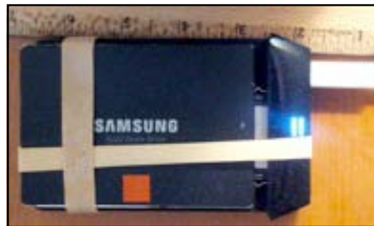
Figure 2: Samsung 840 Pro SSD installed on Thunderbolt adapter.
